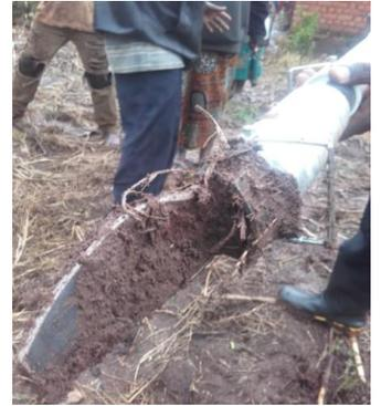
The soils were wet, which caused clogging of the stick. This was the case at both locations. Only on the relatively dry bunds of sweet potato on the light textured soil, the stick worked without interruptions.
