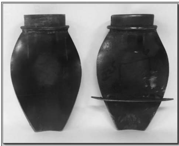
Figure 2. Conventional and tip with a welded stop.
