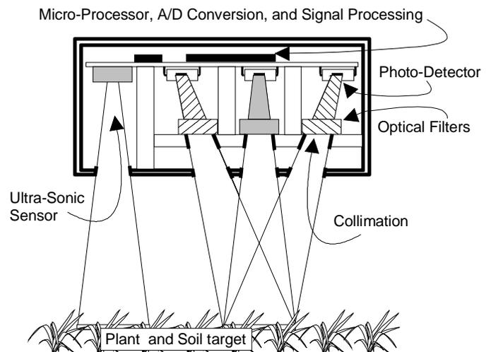
Figure 1. Schematic of the current OSU optical sensor.
