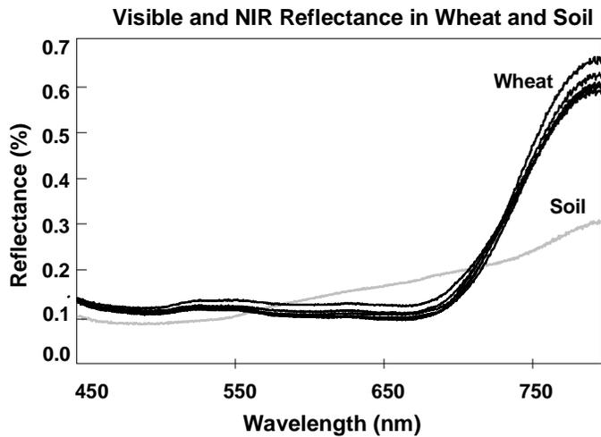
Figure 2. Reflectance in Oklahoma wheat and soil samples
