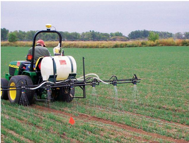
**Fig. 2.** View of the Ramp Calibration Strip applicator showing the boom (3 m wide) capable of delivering 15 different rates at fixed intervals using urea ammonium nitrate via fertilizer stream nozzles.
