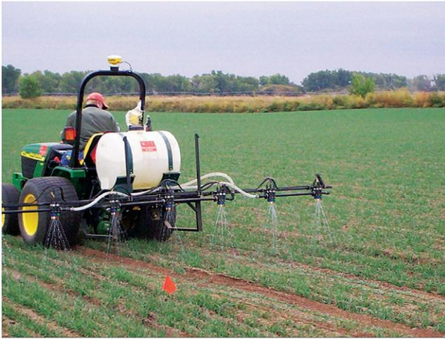
**Fig. 2.** View of the Ramp Calibration Strip applicator showing the boom (3 m wide) capable of delivering 15 different rates at fixed intervals using urea ammonium nitrate via fertilizer stream nozzles.
